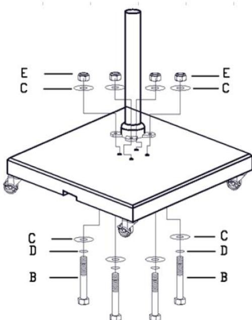
Tools needed for installation; Spanners 13 mm and 14 mm (not included)
